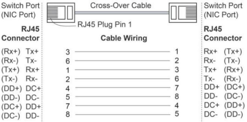
**NOTE** If the PD only supports PoE MDI mode (V+, V+, V-, V- for pins 1, 2, 3, 6), choose a cross-over Ethernet cable to connect the PD and the switch. If the PD only supports PoE MDI-X mode (V-, V-, V+, V+ for pins 1, 2, 3, 6), choose a straight-through Ethernet cable between the PD and the Switch.
