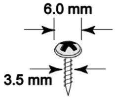
**NOTE** Before tightening the screws into the wall, make sure the screw head and shank size are suitable by inserting the screw into one of the keyhole-shaped apertures of the wall mounting plates. Do not screw the screws in completely—leave about 2 mm to allow room for sliding the wall mount panel between the wall and the screws
