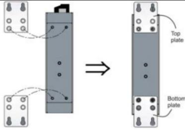
**STEP 2:** Mounting the switch on the wall requires 4 screws. Use the switch, with wall mount plates attached, as a guide to mark the correct locations of the 4 screws. The heads of the screws should be less than 6.0 mm in diameter, and the shafts should be less than 3.5 mm in diameter, as shown in the figure at the right.
