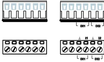
**STEP 1:** Insert the negative (ground)/positive DI wires into the  $\pm$ /I1 terminals, respectively.
