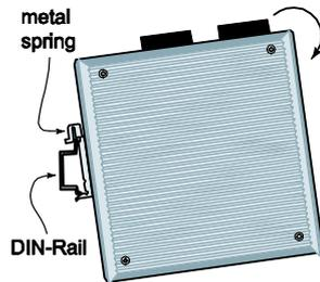
**STEP 2**—The DIN-Rail attachment unit will snap into place as shown in the following illustration.
