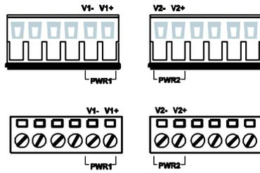
**STEP 1:** Insert the negative/positive DC wires into the V-/V+ terminals, respectively.
